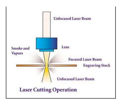
Adjustments can be made to the speed at which the lens moves and the amount of power it discharges. Speed and power settings control the depth of the cut into the material with great precision. This beam is generated from a laser tube and is directed by a series of mirrors, through the lens, and finally onto the laser bed.
