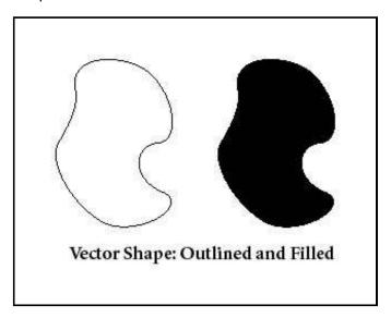
For example, text usually appears on the monitor as filled with black, but its fill can be changed to white and the outline changed from none to black to allow the letters to be vector cut from the material chosen. (It is often necessary for the outline to be assigned a thickness, such as .003" or less, so the laser can vector cut rather than raster engrave the outline. Consult your specific machine documentation for details.)
