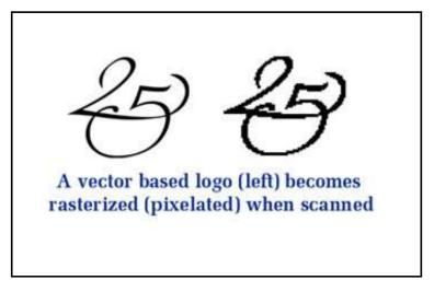
Vector paths can be individual lines or the closed outline surrounding a shape. Vector artwork can be made up of any number of lines or shapes, including text. The laser will move from one line or shape to the next until the artwork is completed. In most cases, the engraving order can be controlled.
