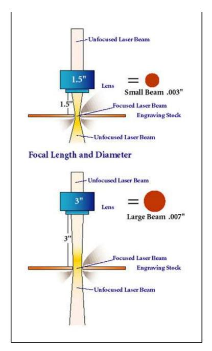
TIP: Since plastic is fairly easy to engrave or cut and is very heat sensitive, a lens with the shortest focal length is the most versatile. Its narrow diameter beam means less heat is concentrated in its path. It also leaves a narrower gap between cutouts when vector cutting and is capable of greater detail engraving.
