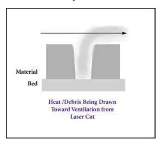
To counter these effects, the smallest focal length lens (smallest diameter beam means less heating area) is recommended together with the minimum combined power and speed settings possible in order to cut through the material. Also lowering the number of pulse firings per inch will keep things cooler. If the PPI is lowered too much, though, the cut edge will start to take on a serrated appearance. In extreme cases, two passes will allow lower combined settings per pass and also minimize damage.
