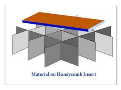
Many engravers use a honeycomb insert, which helps to dissipate heat and debris by raising the material off of the laser bed. This helps but does not eliminate the heat build-up and debris entirely, coming out the top. Others mask the material and wet it down before cutting, which produces good results, but is time consuming.
