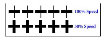
When the laser beam moves across the page, it pulses rapidly whenever it encounters image or text. If the text is small enough, the laser has to turn on and off extremely rapidly which does not give it a chance to burn through fully. By reducing the laser speed, the beam will be able to fully render what is intended. Your laser manufacturer may be able to help remedy this problem; but, in the meantime, decreasing the time setting should resolve it.
